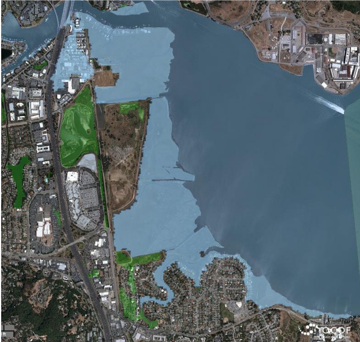
FIGURE 3: FLOODING EFFECT OF 25-CENTIMETER (10-INCH) SEA LEVEL RISE WITH A 20-YEAR STORM
