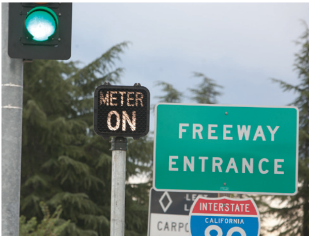
Freeway ramp meter indicator.
